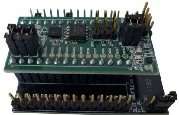
BHI260 shuttle board mounted on level-shifter board (product photo may differ from real product appearance).
